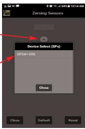
Tap the Reset icon to set the pressure reading to 0 (+/- 0.05 counts)
