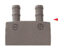
The inputs are marked + and -. Any pressure connected to the - port will be subtracted from the + port. For standard pressure / vacuum measurements use the + port only. Use the + and - port when performing differential measurements.
