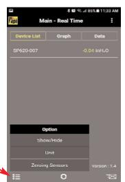
**Show/Hide**: Allows a device to be seen or hidden. Useful when multiple devices are connected.
