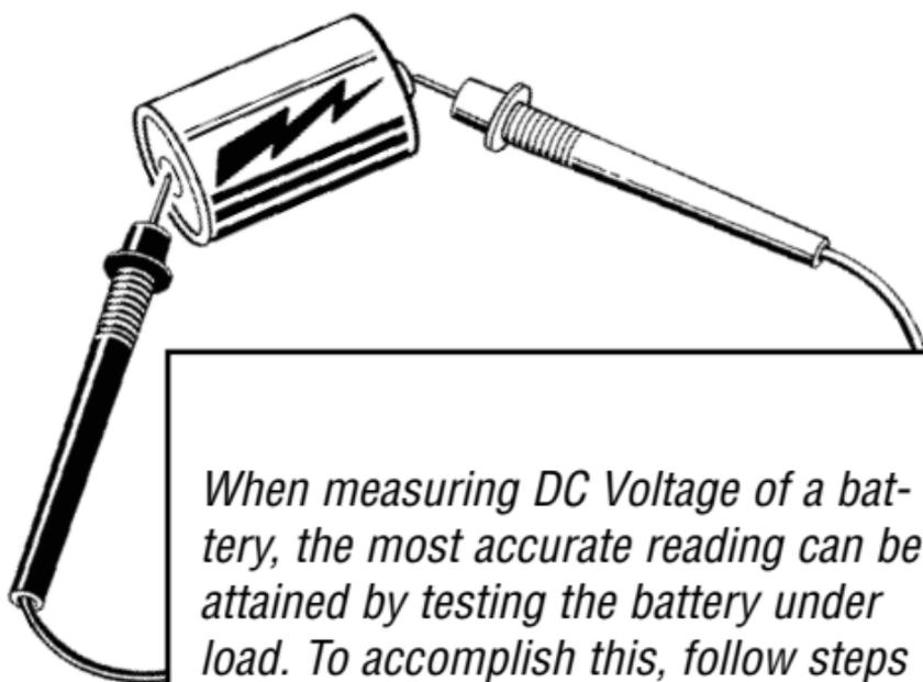
*When measuring DC Voltage of a battery, the most accurate reading can be attained by testing the battery under load. To accomplish this, follow steps 1 through 4 shown on page 14 and the following (with the battery in holder and device turned on):*
